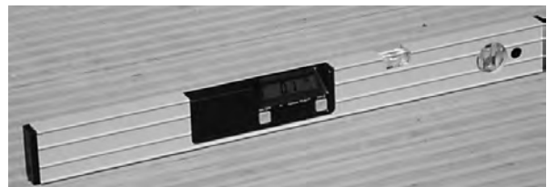
A digital level that can be used with measurements in degrees, percentages, or ratios
