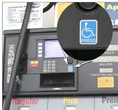
A pump may have a button to notify the attendant that assistance is needed.
